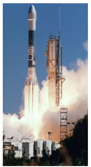
The ELV contains three stages. First and second stages of ELV raise the satellite to an about 50 miles and 100 miles. Third stage of ELV places the satellite in transfer orbit. The task of **ELV** will be completed and its spare parts will be fallen to earth, when the satellite reached to transfer orbit.
