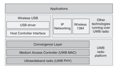
Figure 10-3: Wireless USB Protocol Stack
