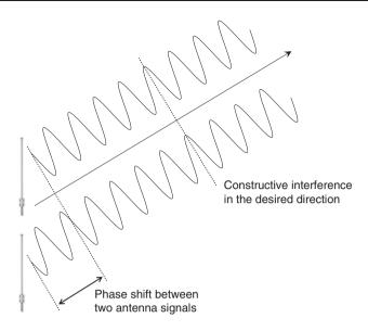
Figure 3-18: Phase Shift Between Two Antennas Resulting in a Directed Beam
