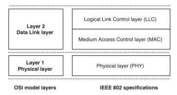
Figure 2-3: OSI Layers and IEEE 802 Specifications
