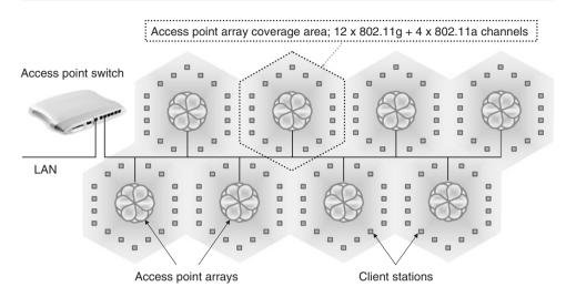
Figure 3-13: WLAN Tree Topology Employing Access Point Arrays
