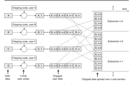
Figure 14-4: Data Spreading in OFDMA/MC-CDMA
