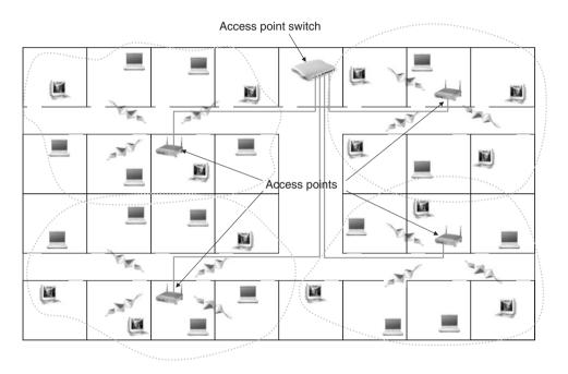
Figure 3-11: Wireless LAN Topology Using a Wireless Switch
