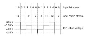
Figure 2-9: 2B1Q Line Code Using in ISDN
