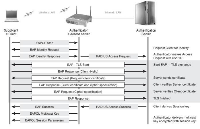
Figure 8-6: EAP-TLS Authentication Exchange
