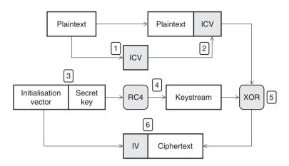
Figure 8-3: WEP Encryption Process
