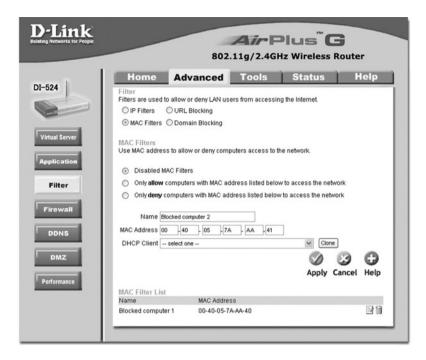
Figure 8-14: Enabling MAC Address Filtering
