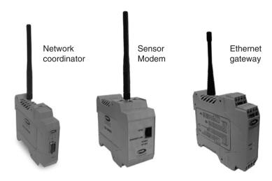
Figure 3-21: A Variety of ZigBee Devices (courtesy of Cirronet Inc.)
