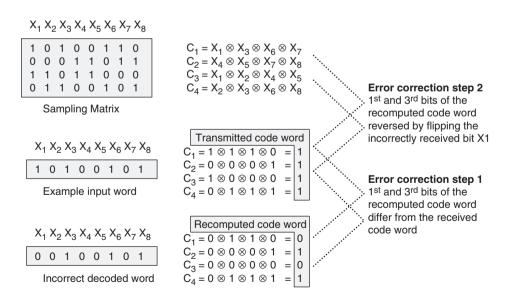
Figure 14-3: LDPC Computation and Error Correction
