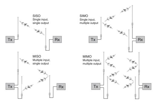
Figure 4-37: MIMO Radio Definition
