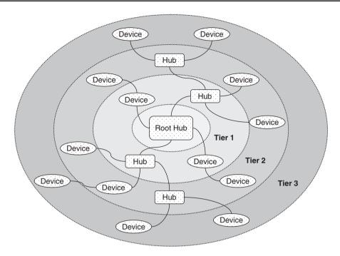
Figure 2-11: USB Network Topology: Daisy-chain and Tree Structures
