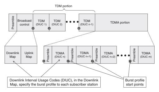
Figure 12-1: 802.16 Downlink Frame Structure
