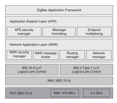
Figure 10-7: ZigBee Outline Protocol Stack
