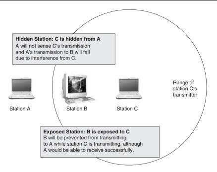
Figure 4-2: Hidden and Exposed Station Challenges for Wireless Media
