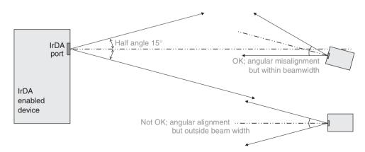
Figure 10-10: IrDA Device Alignment
