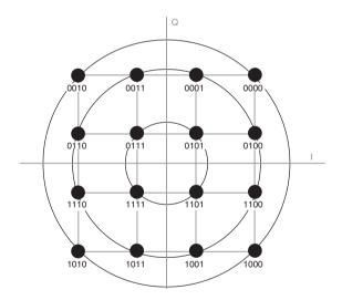
Figure 4-26: Gray Coded 16-QAM Constellation
