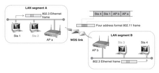
Figure 6-9: Wireless Distribution System Based on Four-Address Format MAC Frame
