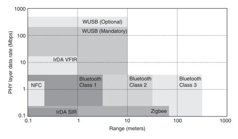
Figure 10-15: PAN Technologies; Range vs. Data Rate
