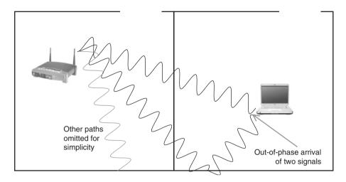
Figure 4-32: Multi-path Fading in an Indoor Environment
