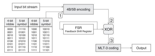
Figure 2-7: 100 Base-T Ethernet Data Encoding Scheme
