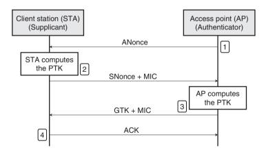
Figure 8-7: EAPoL Key Exchanges of the 4-Way Handshake
