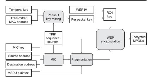
Figure 8-4: TKIP Key Mixing and Encryption Process
