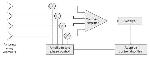
Figure 3-19: Adaptive Beam Antenna
