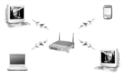
Figure 3-5: Star Topologies in Wireless Networks
