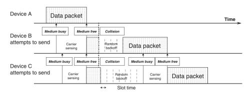
Figure 2-6: Ethernet CSMA/CD Timing
