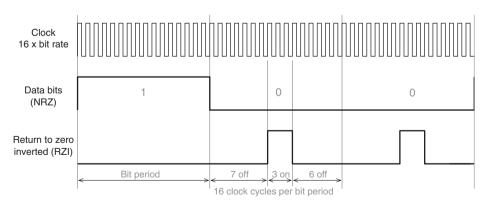
Figure 10-12: IR Pulse Shortening (SIR RZI Modulation)
