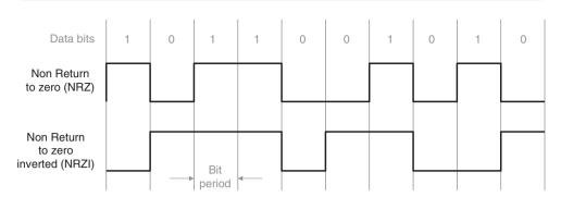
Figure 2-12: USB NRZI Data Encoding Scheme
