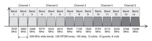
Figure 4-36: MB-OFDM Frequency Bands and Channels
