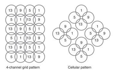
Figure 7-3: Channel Allocation Patterns for Four Non-overlapping Channels
