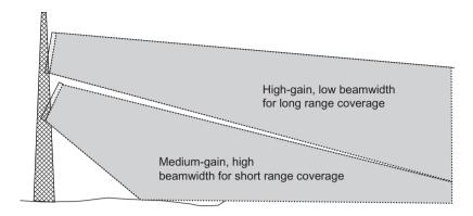
Figure 3-24: WMAN Base Station Sector Antenna Configuration
