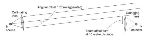
Figure 5-5: Focussed Ir Link Alignment over a 10 m Range
