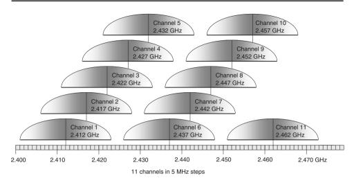
Figure 4-10: DSSS Channels in the 2.4 GHz ISM Band (US)
