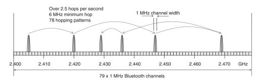
Figure 4-11: FHSS Channels Within the 2.4Ghz ISM Band
