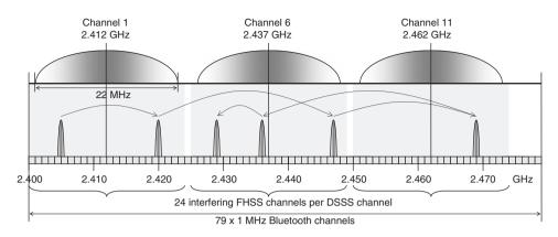
Figure 9-2: Bluetooth and 802.11 DSSS Spectrum Overlap
