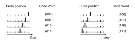
Figure 4-27: 8-PPM Modulation
