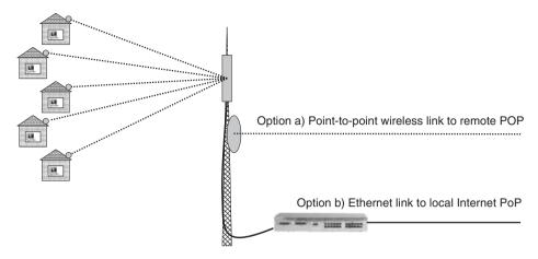
Figure 13-8: Backhaul Configurations
