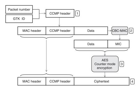
Figure 8-11: MPDU Encryption Using CCMP
