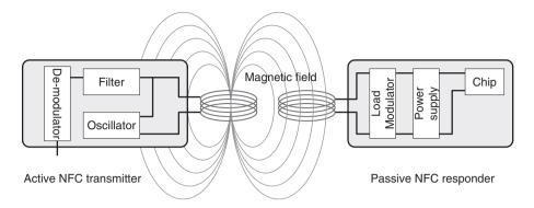
Figure 4-38: Inductive Coupling Between NFC Antenna Loops
