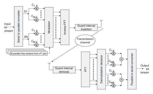
Figure 14-5: Schematic MC-CDMA Transmitter and Receiver
