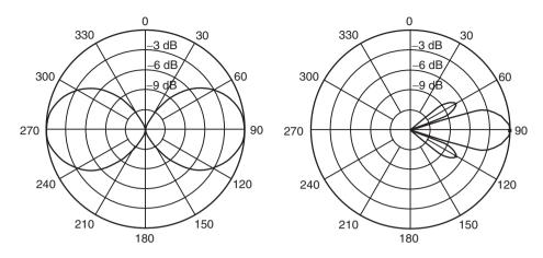
Figure 4-28: Radiation Pattern from Dipole and Yagi Antennas
