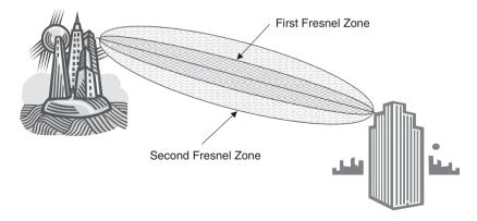
Figure 4-31: The Fresnel Zones Around a Propagation Path
