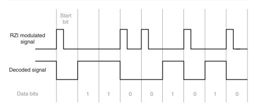
Figure 4-22: RZI Bit Stream Decoding
