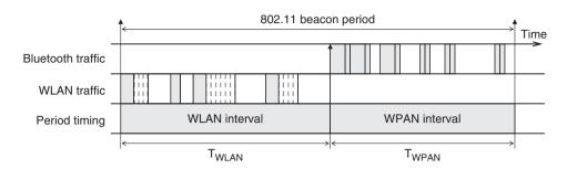
Figure 9-3: WLAN and WPAN Transmit Periods Defined in AWMA
