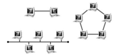
Figure 3-1: Point-to-point, Bus and Ring Topologies
