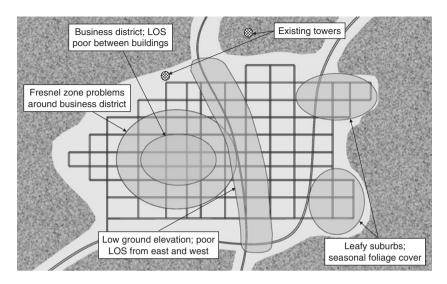
Figure 13-1: A Physical Site-Survey Map for a MAN Installation
