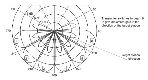
Figure 3-17: Beam Pattern of a Six Element Switched Beam Array
