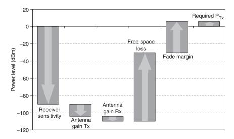
Figure 4-33: Link Budget Expressed as Required Transmitter Power
