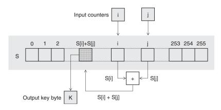
Figure 8-2: Key Stream Generation Using the RC4 Algorithm
