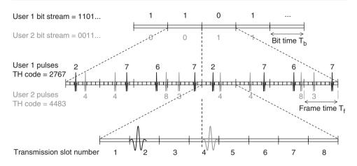
Figure 4-12: Time Hopping Spread Spectrum
