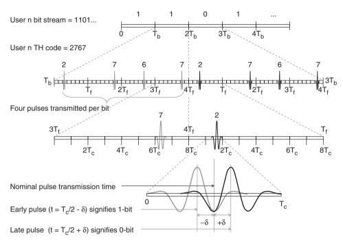
Figure 4-35: Pulse Train in a TH-PPM Impulse Radio Transmission
