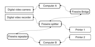
Figure 2-10: FireWire Network Topology: Daisy-chain and Tree Structures
