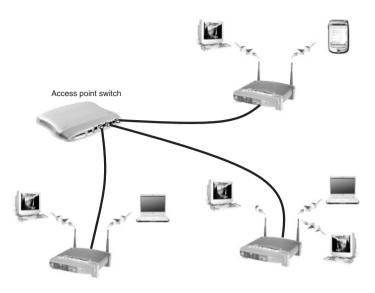
Figure 3-6: A Tree Topology Using a Wireless Access Point Switch
