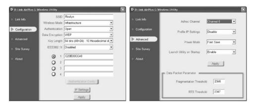
Figure 7-5: Typical Wireless NIC Configuration Screens
