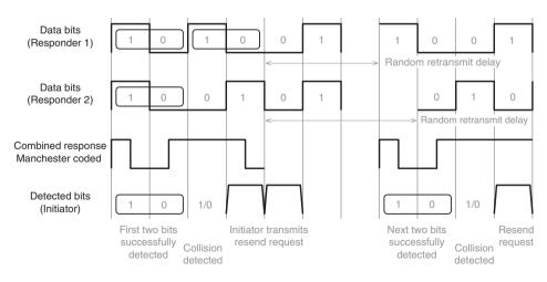
Figure 10-14: NFC Collision Detection with Multiple Responding Targets
