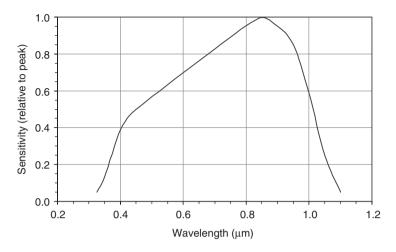
Figure 5-4: Typical Photodiode Sensitivity vs. Wavelength
