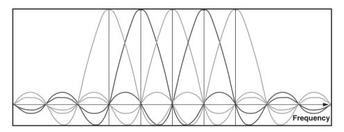
Figure 4-16: Orthogonality of OFDM Subcarriers in the Frequency Domain
