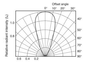
Figure 5-2: Typical LED Emitted Power Polar Diagram
