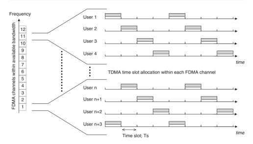
Figure 4-15: FDMA/TDMA Multiple Access System as Used in GSM Cellular Phones
