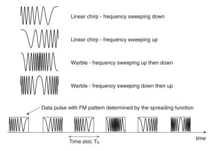
Figure 4-7: A Simple Explanation of Pulsed FM Systems
