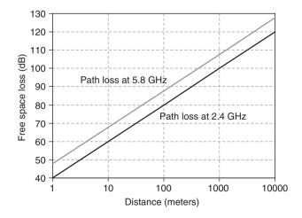
Figure 4-30: Free Space Loss at 2.4 GHz and 5.8 GHz
