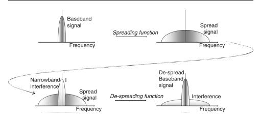
Figure 4-3: A Simple Explanation of Spread Spectrum
