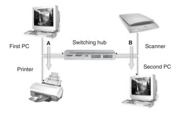
Figure 3-4: Switching Hub in Physical Star Network.
