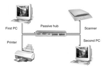
Figure 3-3: A Passive Hub in a Physical Star Network
