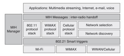
Figure 14-1: MIH Function in the Protocol Stack of a Multi-Radio
