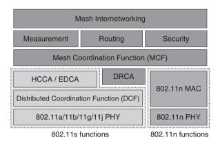
Figure 6-10: Wi-Mesh Logical Architecture
