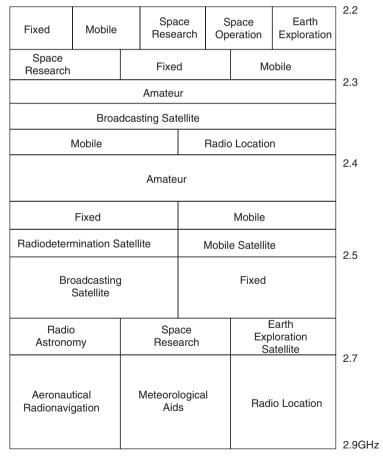
Figure 4-1: FCC Spectrum Allocation Around the 2.4GHz ISM Band
