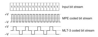
Figure 2-8: Ethernet MPE and Fast Ethernet MLT-3 Encoding
