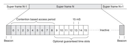
Figure 10-9: ZigBee Superframe Structure
