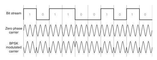
Figure 4-23: Binary Phase Shift Keying Modulation (BPSK)
