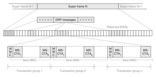
Figure 10-6: Wireless USB Channel within MAC Layer Superframes
