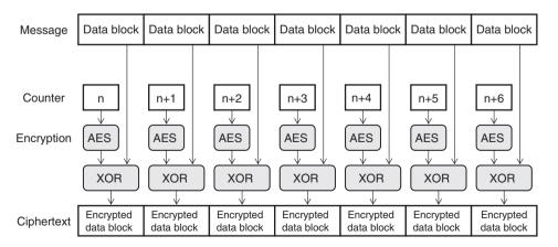
Figure 8-8: Counter Mode of Operation of a Block Cipher (AES)
