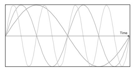
Figure 4-17: Orthogonality of OFDM Subcarriers in the Time Domain
