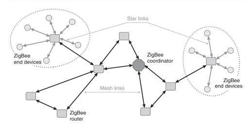
Figure 10-8: ZigBee Supported Topologies
