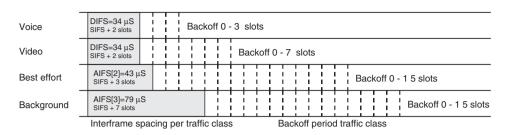
Figure 6-8: AIFS and Backoff Timing per WMM Traffic Class
