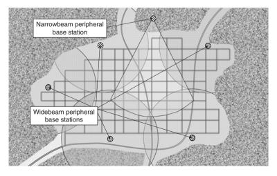
Figure 13-5: Peripheral Coverage of a MAN Target Area
