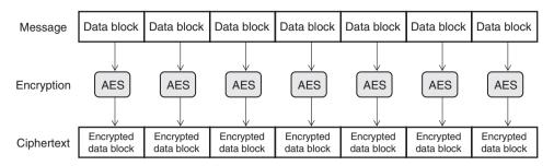
Figure 8-9: Electronic Code Book (ECB) Mode of Operation of a Block Cipher (AES)
