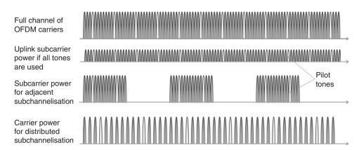
Figure 12-2: WiMax Subchannelization
