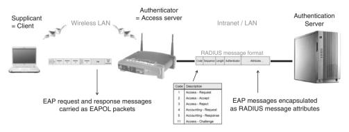
Figure 8-5: Message Format for EAP Over RADIUS Authentication
