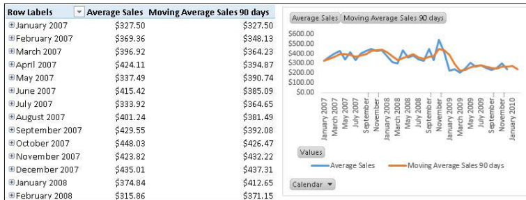
FIGURE 8-8 The line chart compares the simple average for the period selected and the moving average over 90 days.
