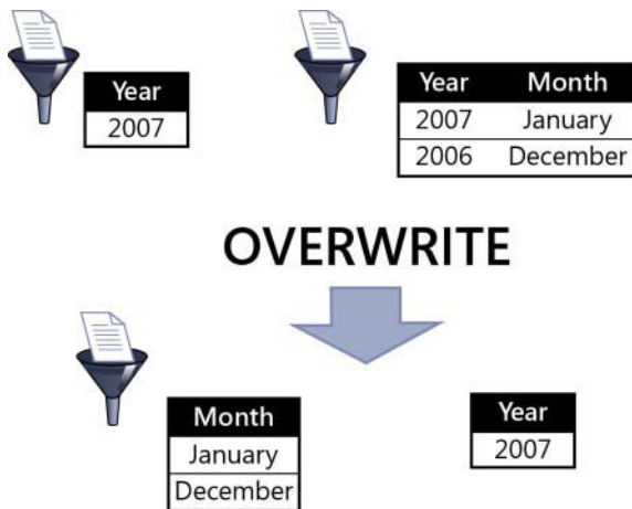
FIGURE 10-30 Applying overwrite to an arbitrarily shaped set might lead to unexpected results.
