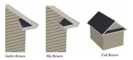
The first two are called **Gable** and **Hip** returns, since the returns themselves end in either a gable or a hip. The third is called a **Full** return because it extends under the entire gable, connecting both sides. Full roof returns are sometimes referred to as water tables.
