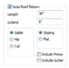
Specify the horizontal **Length** of the returns in inches; the distance to **Extend** the returns past the main roof overhang; the style of roof return; and whether the returns are sloping or flat. As long as your model has a roof, the specified roof returns will be generated when you click **OK**. For more information, see "Roof Returns" on page 480 of the Reference Manual.
