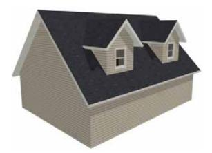
8. Notice there are small gaps in the dormer side walls. This gap is caused by the difference between the position of the knee walls and the point at which the ceiling intersects the roof plane. This location is marked by the black dotted line in floor plan view.
