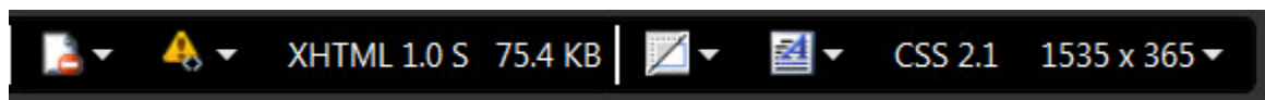
Figure 58: Status Bar From L to R, the symbols: Incompatible HTML - Invalid HTML - HTML schema - File Size - Visual Aids Mode - CSS schema - Current Page size
